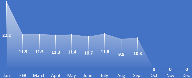
WELL # 11 PUMPING LEVEL TO SHUTOFF
